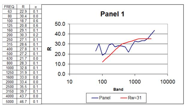
NOTES R – Sound transmission loss in one  $1/3^{rd}$  octave band;  $\sigma$  – standard deviation
