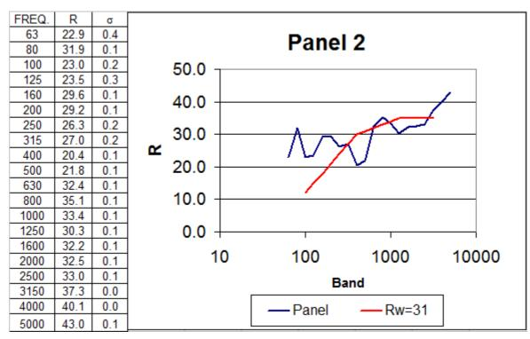
NOTES R – Sound transmission loss in one  $1/3^{rd}$  octave band;  $\sigma$  – standard deviation
